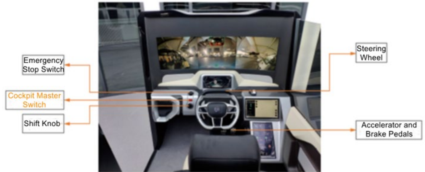
Unity Drive's remote cockpit (ultralow latency: \leq 50\text{ms} )
