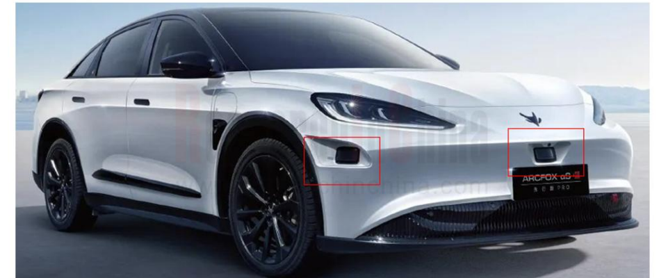
ARCFOX αS Advance Edition PRO Equipped with 3 LiDARs
