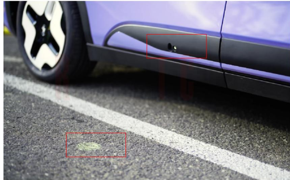
ARCFOX Kaola Sliding Door Opening by AR Projection
